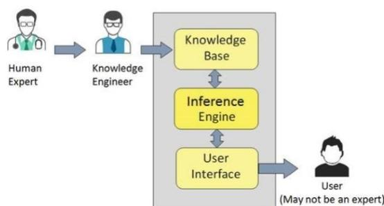
**Figure1:** General Structure of an Expert System[6]
