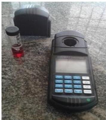
**Figure S3.** DR-850 Colorimeter- Instrument used for the quantification of fluoride in treated
