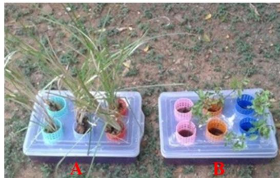
**Figure S2.** Hydroponic System for the determination of defluoridation efficiency of *Chrysopogon zizanioides* (A) and *Ocimum tenuiflorum* (B).
