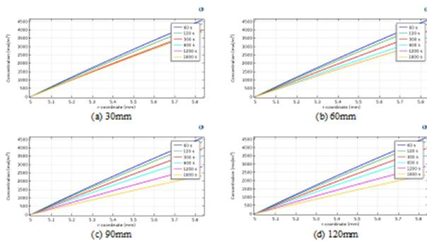
**Fig. 15** Concentration distribution of water in membrane phase ( $C_{\text{water-membrane}}$ ) at different heights (1 l/min feed flow rate and  $30^\circ\text{C}$  temperature); (a) 30mm, (b) 60mm, (c) 90mm and (d) 120mm
