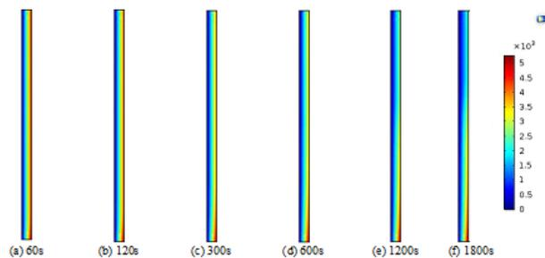
**Fig. 14** Concentration distribution of water in membrane phase ( $C_{water-membrane}$ ) at different separation times (1 l/min flow rate and 30°C temperature); (a) 60s, (b) 120s, (c) 300s, (d) 600s, (e) 1200s and (f) 1800s
