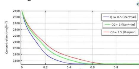
**Fig. 17** Concentration distribution of water in membrane phase ( $C_{\text{water-membrane}}$ ) vs. dimensionless height at different feed flow rates
