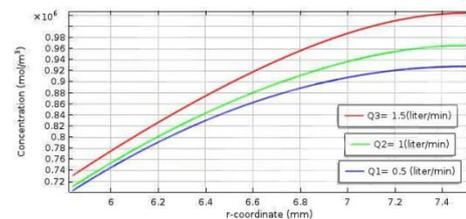
**Fig.13** Water concentration distribution in feed phase vs. radius at 30°C temperature and various feed flow rates
