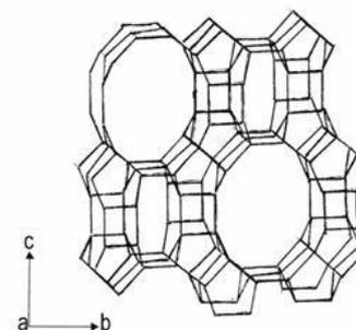
Fig. 1 Schematic representation of mordenite structure
