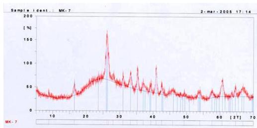
Fig. 6 XRD pattern of the mordenite zeolite membrane
