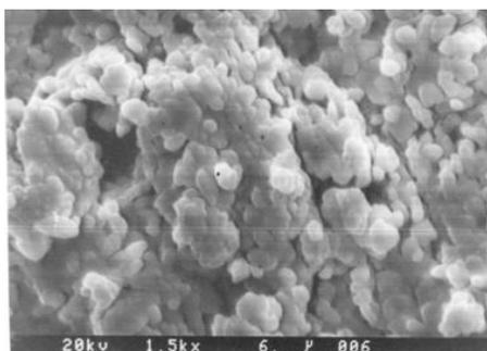
Fig. 7 SEM of the mullite support
