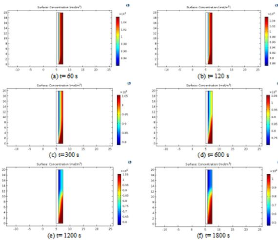
**Fig. 9** Concentration distribution of water in feed phase ( $C_{water-feed}$ ) at different times (1 l/min flow rate and 30°C temperature); (a) 60s, (b) 120s, (c) 300s, (d) 600s, (e) 1200s and (f) 1800s
