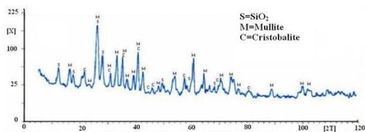
Fig. 5 XRD pattern of the mullite support
