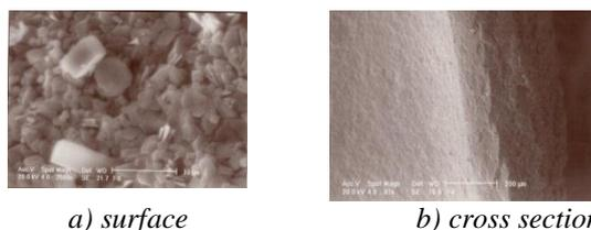
Fig. 8 SEM of the mordenite zeolite membranes
