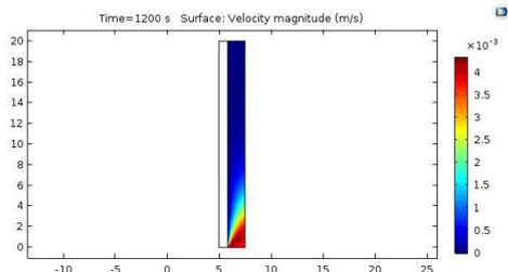
Fig. 19 Velocity distribution in the feed phase at 1 l/min feed flow rate and 30°C temperature
