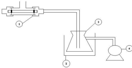
**Fig. 2** PV setup; 1- feed container and PV cell 2- liquid nitrogen trap 3- permeate container 4- three stage vacuum pump
