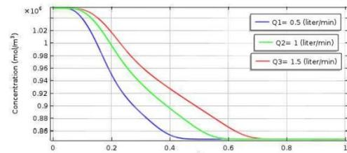
**Fig.12** Water concentration distribution vs. dimensionless height in feed phase at 30°C temperature and various feed flow rates
