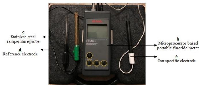
Figure (1): A microprocessor based portable fluoride meter.
