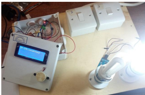
Figure 9. System Testing 36W and 45W CFL
