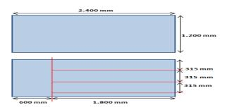
Figure 1. Plate before and after cutting
