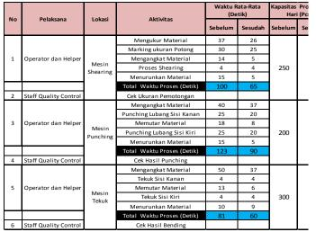
Table 3. Comparison of processing time before repair and estimationaverage process time after repair
