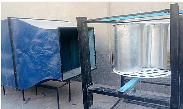
Figure 1: Experimental rig with Savonius rotor model
