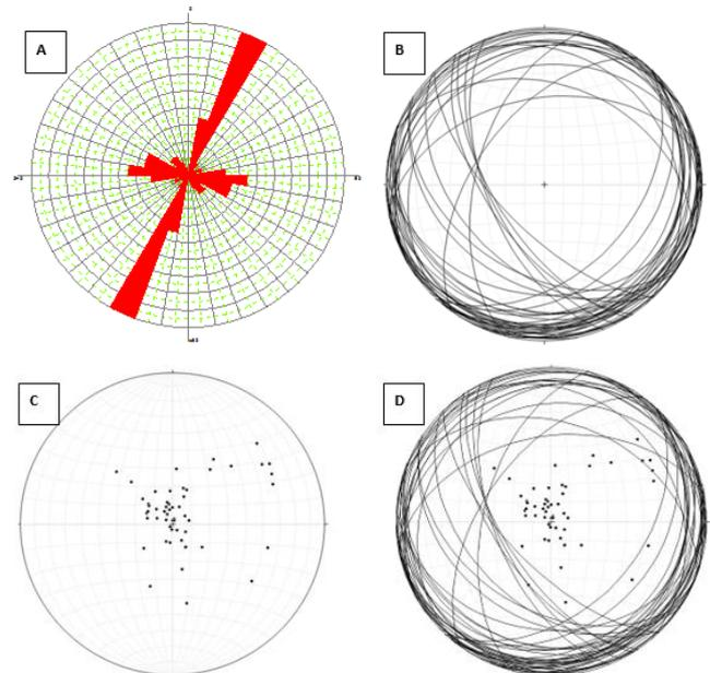
**Figure 9:** A: Rosette plot for dykes and veins. B: Beta diagram for attitudes of foliation planes. C: S-pole for attitude of foliation planes. D: Combined Beta and S-pole diagrams for attitude of foliation planes.
