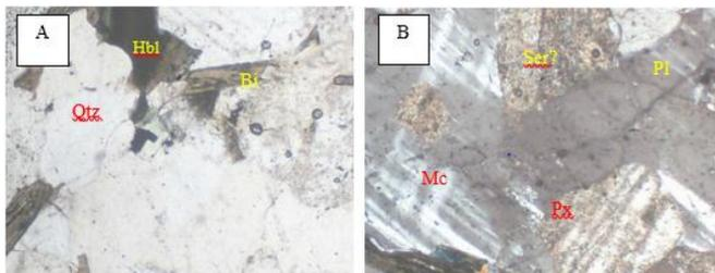
**Figure 5:** Photomicrograph of granitic gneiss (magnification =  $\times 20$ ) under A: Plane polarized light B: Cross polarized light
