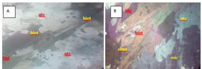
**Figure 7:** Photomicrograph of migmatite gneiss subplanar alignment of prismatic minerals and stretched quartz grains (magnification =  $\times 20$ ) under A: Plane polarized light. B: Cross polarized light.
