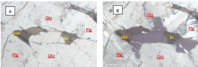
**Figure 4:** Photomicrograph of Biotite hornblende granite (magnification =  $\times 20$ ) under A: plane polarized light. B: cross polarized light
