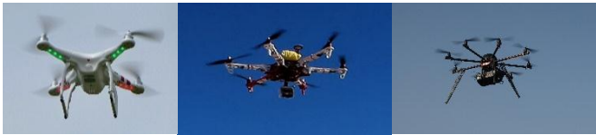
Figure 1: Examples of rotocopter UAVs. From left to right: quadrotor (quadcopter), hexacopter and octocopter [2], [3]. Another type of rotocopter, the helicopter, is not shown.
