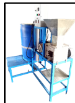
Figure 1. Final Set-up of the Chitin Extracting Machine
