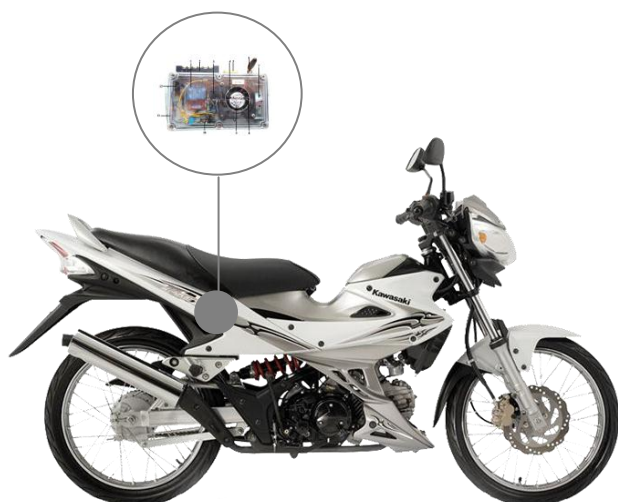
Figure 5. Installation of the device in the motorcycle u-box
