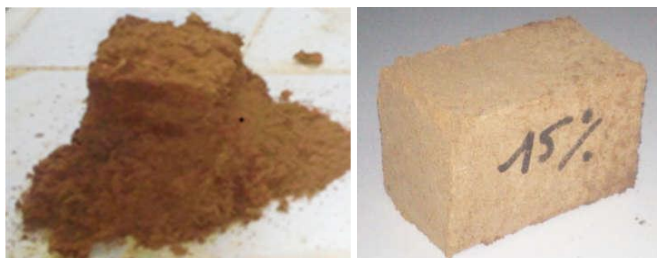
c) test tube 10% latex d) 15% latex test tube
