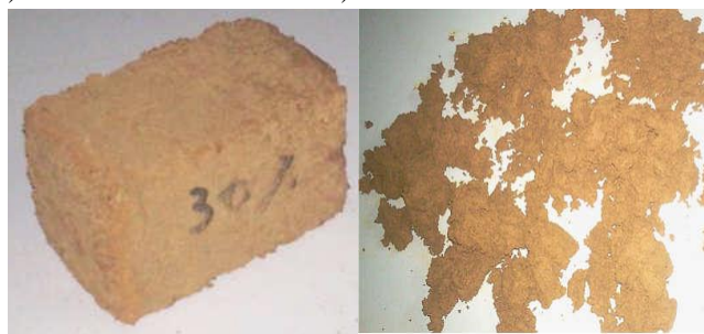
g) test tube with 30% latex h) rubbery sample with 35% latex
