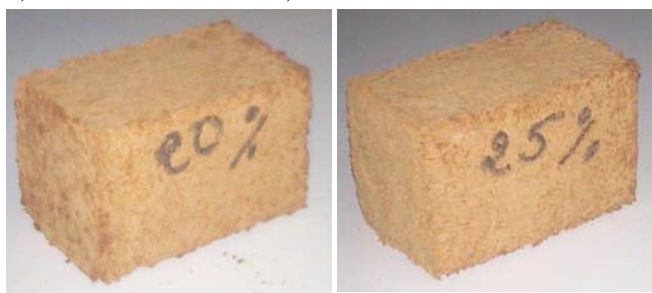
e) test tube with 20% latex f) test tube with 25% latex
