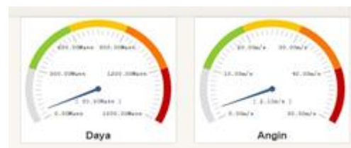
Figure 10. Display of power and wind monitoring
