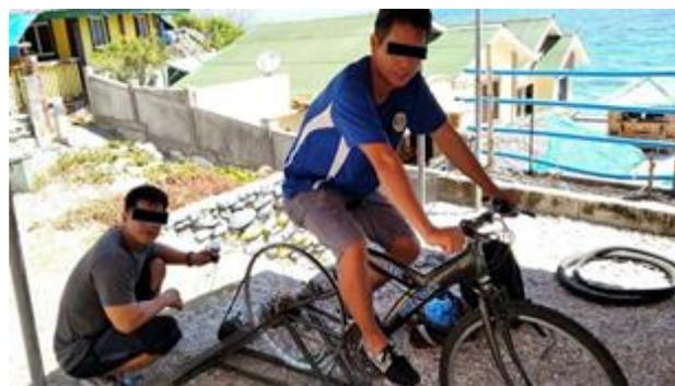
**Figure 4:** Pedal-powered alternator installed at Isla Verde, Batangas
