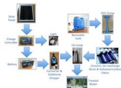
*Figure 1: Operation diagram of Water-Electricity-Light System*
