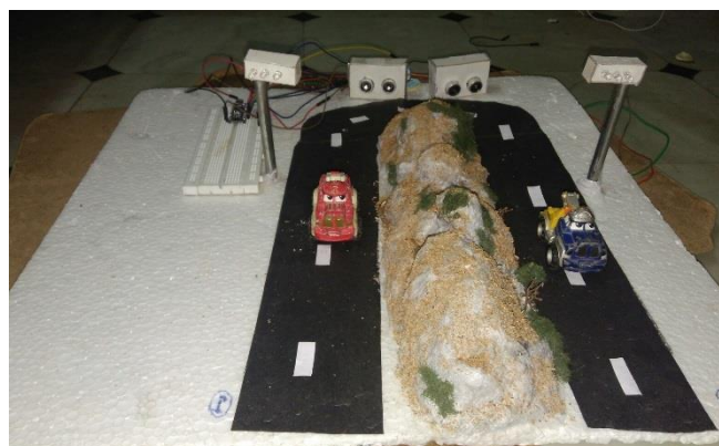
Fig 9: Model setup of Ultrasonic sensor and Arduino on a curved road.
