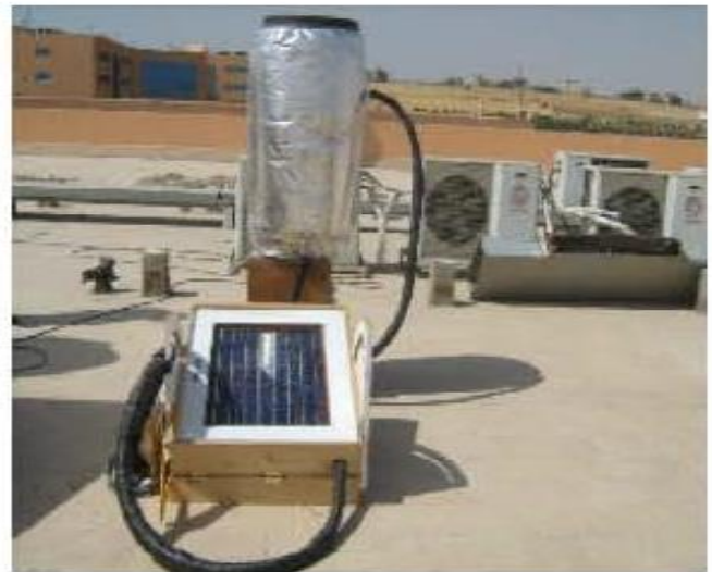
Figure-6: Thermo-syphon effect used on PV/T system [36]
