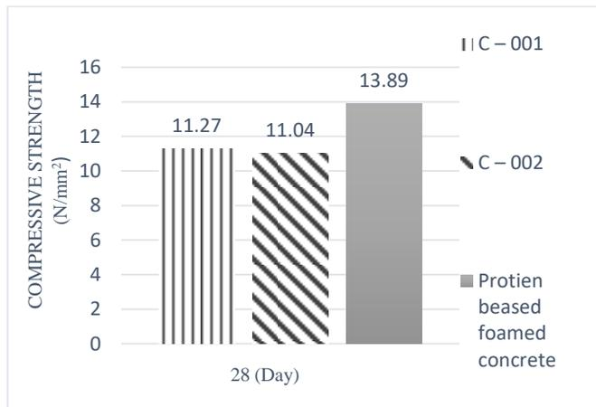
**Figure 2:** Variation of Compressive Strength with Age for C- 001, C- 002 and the Protein Based Foamed Concrete.
