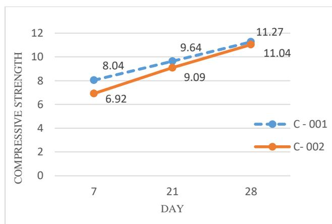
**Figure 1:** Variation of Compressive Strength with Age for C-001 and 002
