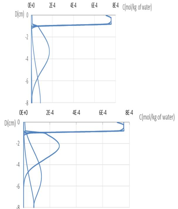
Figure 13: concentration of contaminant (C) in the soil profile (a)CEC=0.5 (b)CEC=0.1
