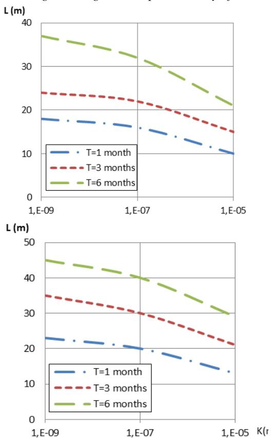
Figure 8: Length variations of contamination in fine soils according to changes in the permeability of the soil
