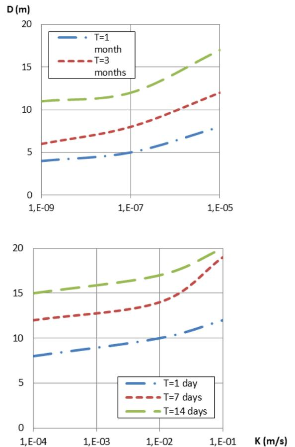
Figure 7: Depth variations of contamination in coarse soils according to changes in the permeability of the soil
