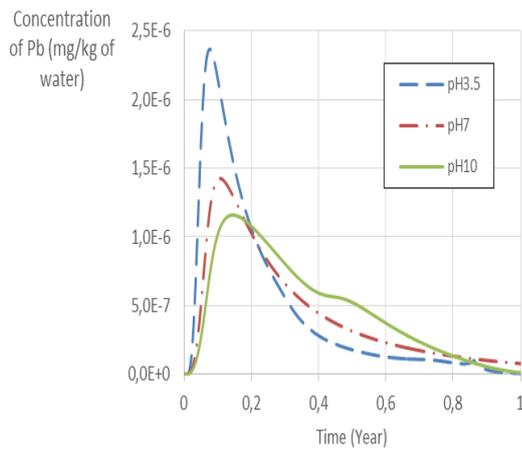
Figure 11: Output concentration of Pb from soil column
