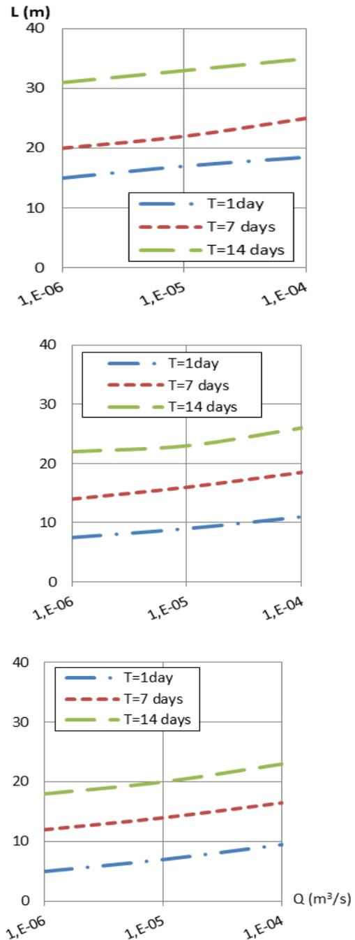
**Figure 10:** Length variations of contamination in fine soils according to changes in the inflow discharge of the contaminant in coarse soils with different permeability
