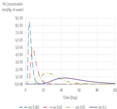
Figure 12: Pb concentration in the soil with different ion exchange capacity
