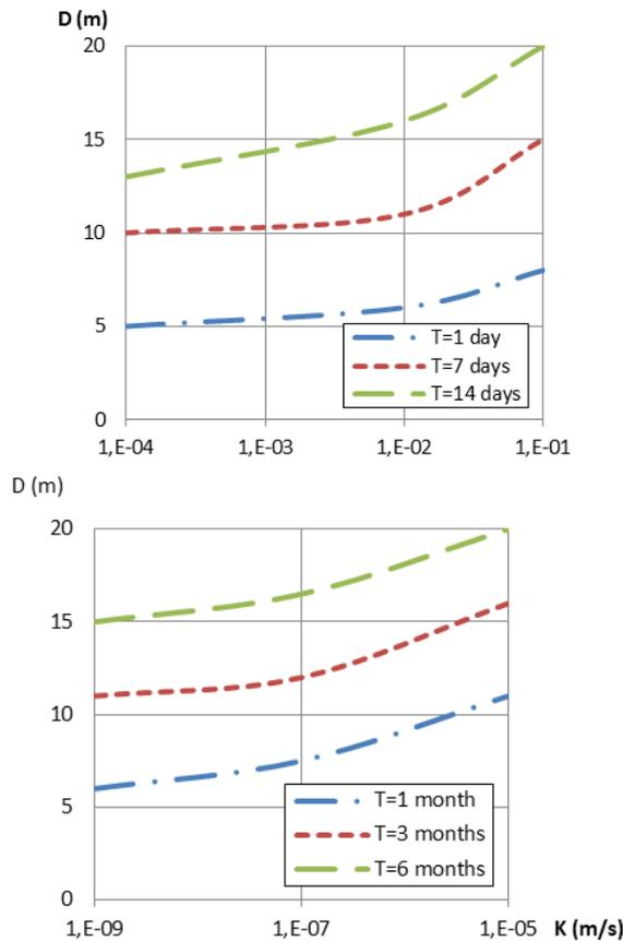
**Figure 9:** Depth variations of contamination in fine soils according to changes in the permeability of the soil
