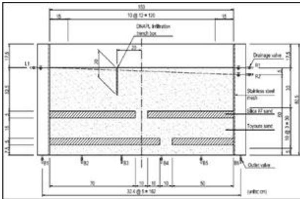
Figure 2: The diagram of intermediate-scale container for oil movement tests.
