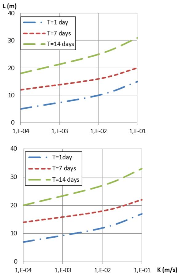
Figure 6: Length variations of contamination in coarse soils according to changes in the permeability of the soil
