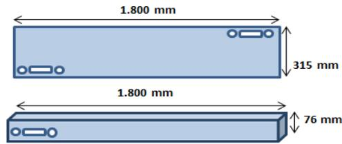
Figure 3. Plate before and after bending
