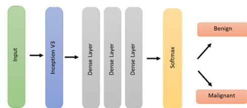
**Figure 6:** High Level overview of architecture of our neural network with Google’s Inception-v3 included inside it. The input image is fed into the 1<sup>st</sup> layer of Inception-v3. The final layer of inception-v3 is removed and 3 fully connected layers were added followed by a Softmax layer. In this way, we could be able to tune Inception-v3 according to our problem statement.
