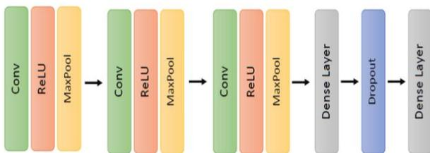
**Figure 4:** Architecture of Simple Convolutional Neural Network that was mainly for preliminary viewing of output result. The network contains 3 convolution layers each followed by Max-Pool operation and ReLU activation function and two fully connected layer at the end with proper dropout.
