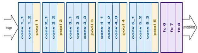
**Figure 5:** Architecture of further deeper and denser neural network developed after improving 1<sup>st</sup> model. Convolutional Layers has been increased followed by 3 fully connected layers, and thus making the network similar to VGGnet.
