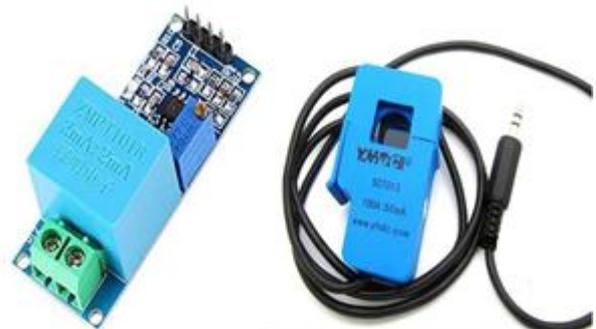
Figure 4. ZMPT 101 voltage sensor and SCT-013 101 current sensor in the monitoring system
