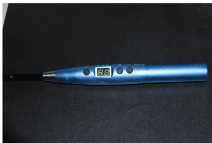
Figure 3: light curing unit.
